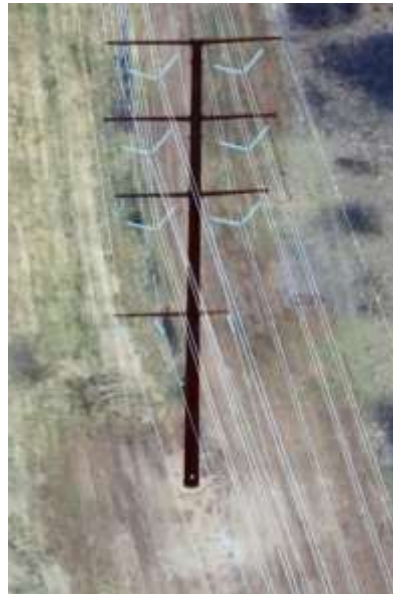
Double-Circuit Running Angle
